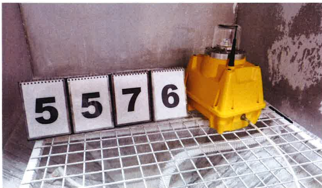
Fig. 2. Test sample 5576 in the dust chamber – before the IP6x test.
