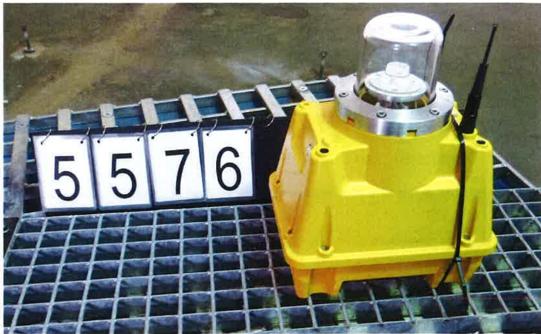
Fig. 1. Test sample 5576 – before the IPx7 test.
