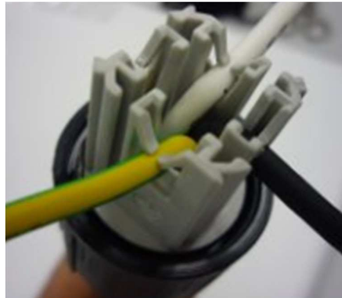
Figure 27: wires fitte-in – top view
