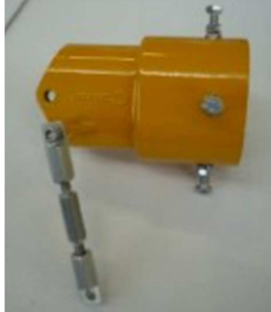
Figure 12: support with vertical aiming adjusting device
