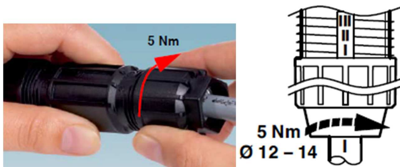
Figure 13: tightening torque
