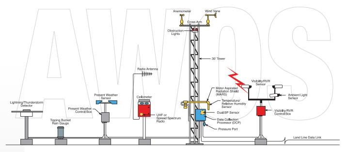
Within the architecture of the AWOS System is the most advanced Data collection platform and Central data computer available today. This creates the most flexibility with data displays single and multiple display options. All ANS AWOS systems have remote capabilities so that we are able to support you from afar.
