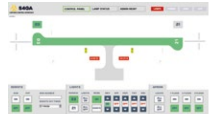
AGL CONTROL AND MONITORING
